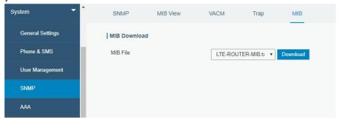
2. Start "ManageEngine MibBrowser Free Tool" on the PC. Click "File > Load MIB" on the menu bar. Then select "LTE-ROUTER-MIB.txt" file from PC and upload it to the software.
