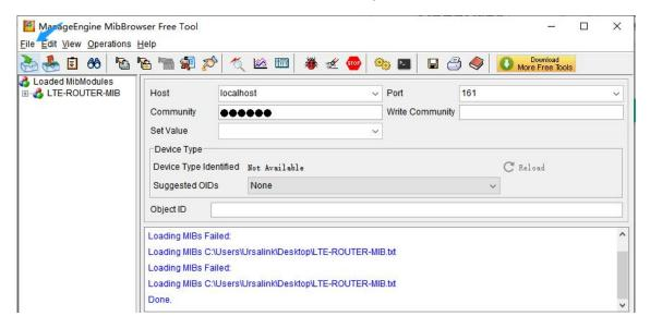
Click the "+" button beside "LTE-ROUTER-MIB", which is under the "Loaded MibModules" menu, and find "usCellularinfo". And then you will see the OID of cellular info is ".1.3.6.1.4.1.50234", which will be filled in the MIB View settings.
