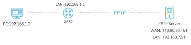
Configure the UR32 as PPTP client to connect to a PPTP server in order to have data transferred securely. Refer to the following topological graph.
