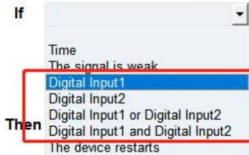
The user can setup multiple combinations; however, input 1 and input 2 must be activated before action is taken.
