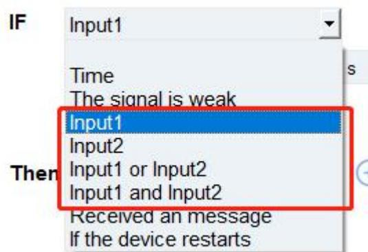
The user can setup multiple combinations; however, input 1 and input 2 must be activated before action is taken.
