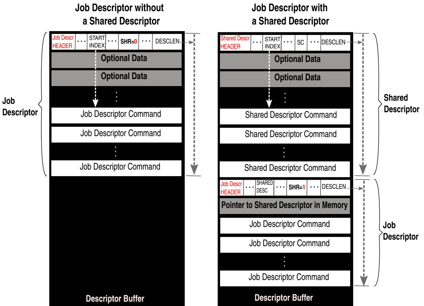
Figure 10-8. Job Descriptor layout in descriptor buffer
